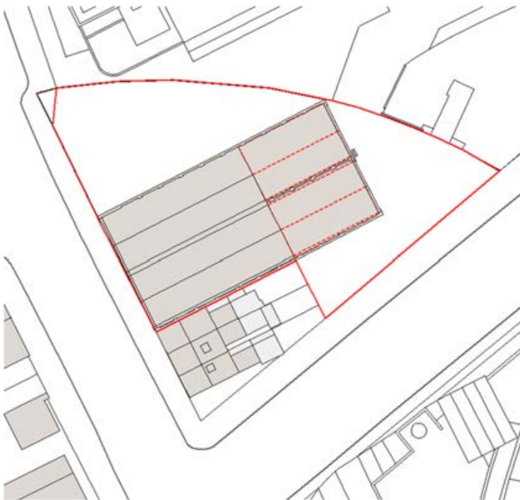
Figure 110 – demolition plan for 12 Pyrmont Street
